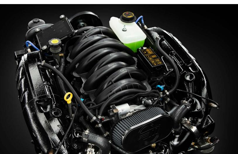
Although the Axis fuel system works very efficiently, there will always be some gaseous by-product as a result of operating an internal-combustion engine. These gases, along with the water used to cool the engine (in addition to the closed cooling system) are routed out of the boat by way of the exhaust manifolds on each side of the engine to exhaust houses between the deck and hull, and it is expelled out of the system at the transom.
