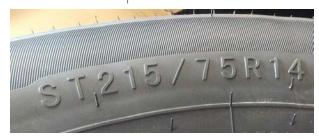
ST: The ST indicates that the tire is for trailer use. Next number: This three-digit number gives the width in millimeters of the tire from sidewall edge to sidewall edge. In general, the larger the number, the wider the tire.
