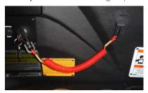
lanyard to the switch on the shifter/throttle, and to a piece of the operator's clothing.
