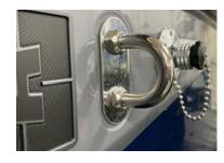
eyes (along with the transom grab handle and/or the tower tow point) are used to tie-up the boat, and no other part of the boat, including any interior components such as the windshield extrusions or grab handles should ever be used.
