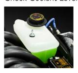
Be certain the emergency safety stop switch is disconnected, and the shifter/throttle is in neutral. Open the engine compartment hatch and locate the coolant reservoir. The reservoir will be located on the port side of the engine between the
