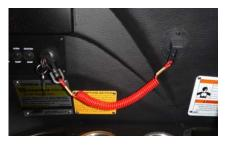
will not start and/or run if the toggle is in the OFF position. Axis recommends the clip always be inserted in the toggle switch. Connected to the operator, if (s)he moves away from the controls, the clip will pull free, pulling the switch to the OFF position. If the engine needs to be shut down very quickly, it can be done so by pulling on the lanyard to release it from the switch. To reset the switch after activation, reinstall the lanyard clip and flip the switch to the UP position.
