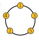
star pattern; do not simply go around clockwise or counterclockwise. The cross effort will ensure a correct reading.
