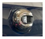
visibility. There is a green light on the starboard side and a red light on the port side, operated from a button on the dash panel. The green light will be on the starboard side of the deck adjacent to the driver's helm, and the red light will be on the port side deck adjacent to the observer seat location. The lights are controlled from a button on the dash panel.
