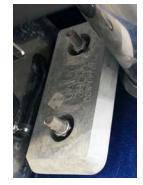
transom zinc anode via grounding wire. Anodes are also affixed to the exhaust manifolds.
